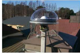
Figure 2. Left: Sketch of the pillar top at the fundamental SWEPOS stations with an attached GNSS antenna and covered by a radome. Right: Photo of a typical roof-top mount.
