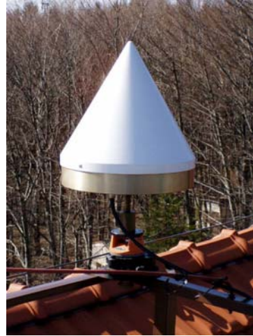
Fig. 2 – Topcon CR3 GGD antenna on metallic barrier
